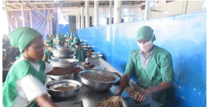
After cashews have been through an automatic shelling machine, Tolaro Global staff manually check them and unshell those missed. Photo credit: Tolaro Global
